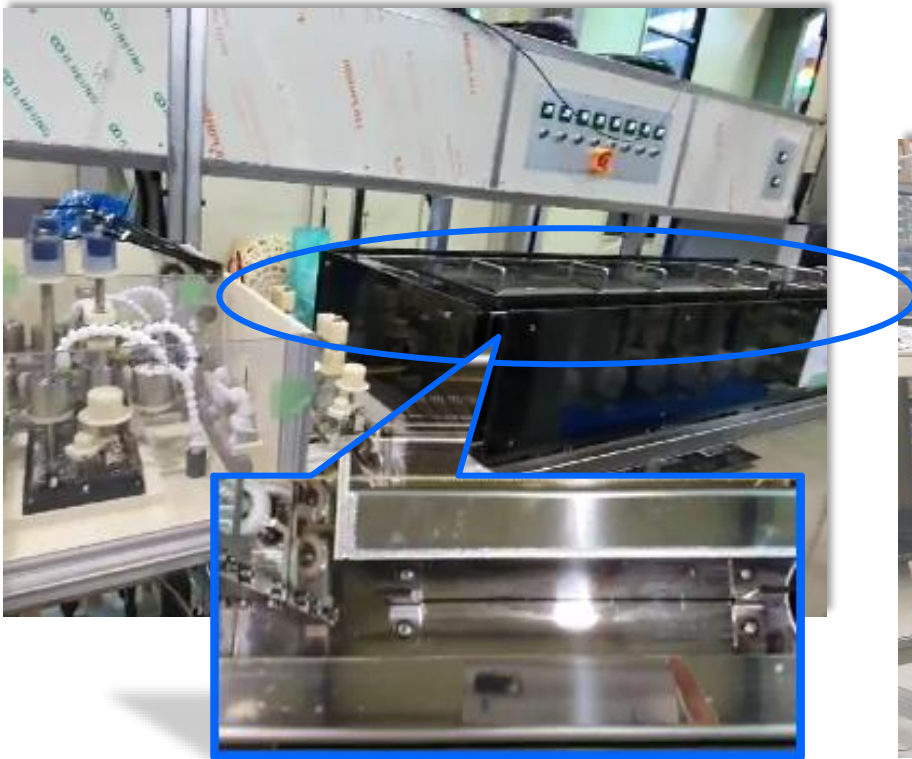
Sn-Connector Reflow 상부 CELL
